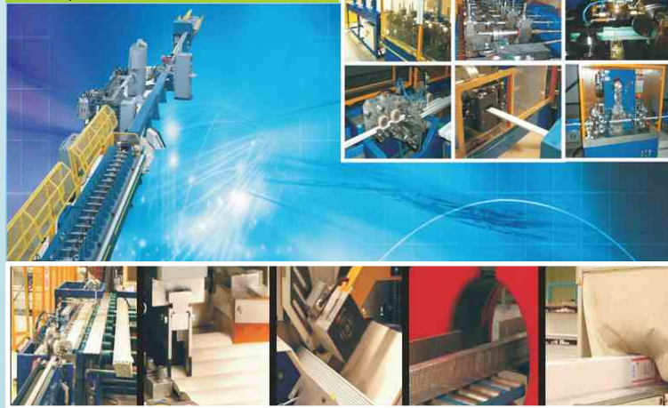
Aluminium slat with poyurethane inside production line
